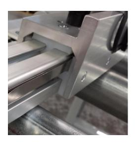
Reinstall your carriage with the scale facing the back of the carriage as shown.
