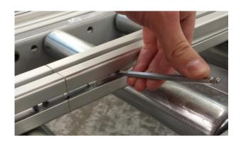
Continue tightening the bolt until the butt splice is tight. Make sure the extrusion sections are aligned as you tighten the butt splice.
