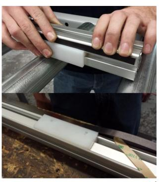
Clean the rail with acetone or isopropyl alcohol to remove any residual oil and debris. Now, begin to remove the adhesive backing from the scale and press it firmly against the rail. Rest the scale against the guide and work your way down the rail, installing the scale.
