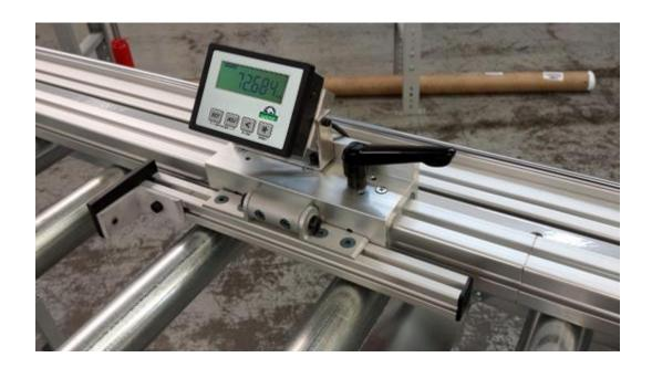
Do not install the scale until the splice is adjusted and the rail is final mounted. The scale can not be removed to adjust the splice later. If the rail is not final mounted to fully support the splice, issues could arise from the scale shifting, if the splice is allowed to flex.
