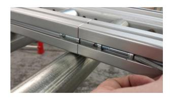
Slide the bolt toward the butt splice hardware and begin threading it into the opposing butt splice.
