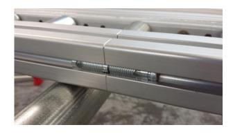
It is important that the rail is mounted to a flat surface to ensure the rail sections remain square. This will allow the carriage to move freely over the splice.
