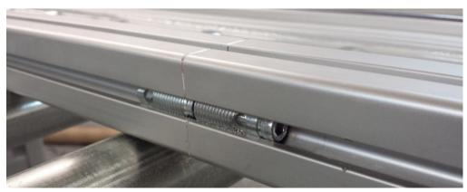
The rail is marked to indicate the location on the rail that the scale is to be installed. (Note: The scale and steel cover strip are not directional). Use the included UHMW guide to ensure the scale is installed straight and in the correct location.
