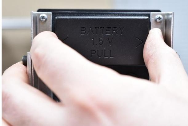
With the cover removed, you can see that the battery is held in by two plastic fingers, one on top and one on the bottom.
