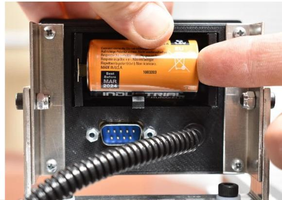
Pivot the battery from the negative end until it clears the plastic fingers and can be fully removed.
