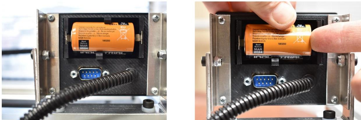
Pivot the battery from the negative end until it clears the plastic fingers and can be fully removed.
