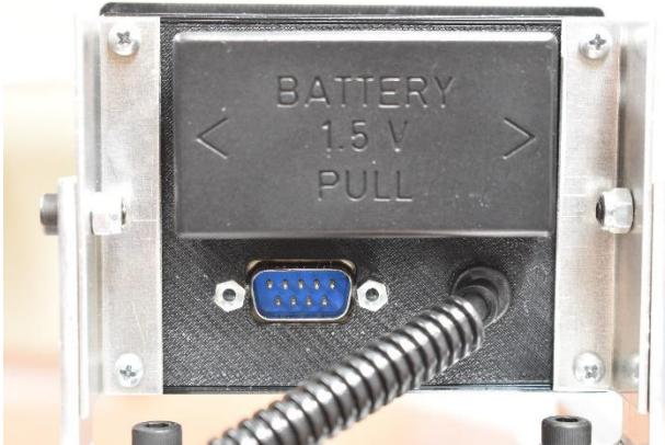
Your DRO is equipped with an RS232 port below the battery compartment. This port allows you to export data directly from your DRO to your computer via one of two optional SPC accessories. Hymark offers both wireless and wired SPC accessories that enable the SPC output function of the MMP to transmit data to a PC by pressing **SET**. For more information or to purchase one of these devices please visit our website at [kentuckygauge.com](http://kentuckygauge.com).
