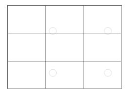
The grid to the left divides your MMP jaw in to 9 sections. Take a measurement at the center of each of these sections, being sure not to take measurements with your ball gage in one of the mounting screw holes.
