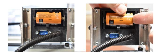
Pivot the battery from the negative end until it clears the plastic fingers and can be fully removed.
