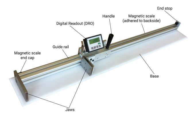
Note: DRO is powered by (1) C battery. The battery will need to be replaced approximately every 9-12 months depending on use and battery capacity. An industrial grade battery is recommended for maximum battery life.
