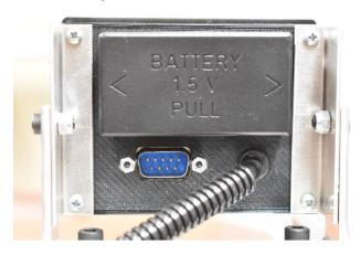
Your DRO is equipped with an RS232 port below the battery compartment. This port allows you to export data directly from your DRO to your computer via one of two optional SPC accessories. Hymark offers both wireless and wired SPC accessories that enable the SPC output function of the MMP to transmit data to a PC by pressing SET. For more information or to purchase one of these devices please visit our website at kentuckygauge.com.
