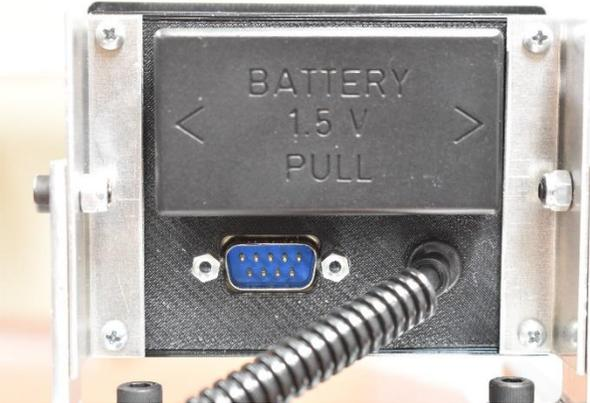
Your DRO is equipped with an RS232 port below the battery compartment. This port allows you to export data directly from your DRO to your computer via one of two optional SPC accessories. Hymark offers both wireless and wired SPC accessories that enable the SPC output function of the MMP to transmit data to a PC by pressing . For more information or to purchase one of these devices please visit our website at [kentuckygauge.com](http://kentuckygauge.com).
