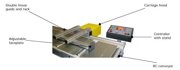
Note: Carriage length and depth can differ depending on motor and gearbox type
