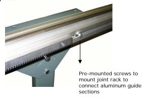
Mount joint rack to 1<sup>st</sup> aluminum guide section by using the short adapter rack piece, the two metal spacers and a clamp
