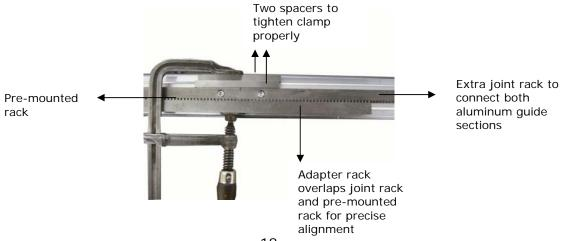
Tighten all socket head cap screws of the joint rack on 1<sup>st</sup> aluminum guide section
