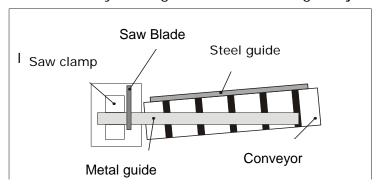
Adjust the conveyor so it is leveled lengthwise using a metal guide set in the saw clamp.
