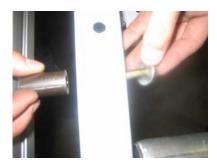
Note: Do not tighten the screws at this point to be able to align the T-nuts with the conveyor mounting holes and to align the aluminum extrusion in X direction when mounted to the conveyor
