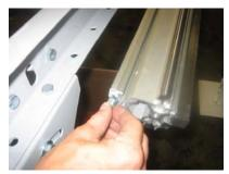
Mount aluminum extrusion to conveyor by using M8 socket head cap screws with washers and stand-offs. Stand-off length is designed for Kentucky Gauge conveyors series RC and RH.
