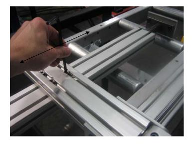
Adjustable stop arm in X, Y & Z direction
