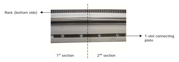
Tighten now all socket head cap screws that connects conveyor with  $2^{nd}$  aluminum guide section
