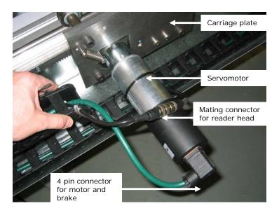
Unscrew motor set screw to be able to push down motor with spur gear
