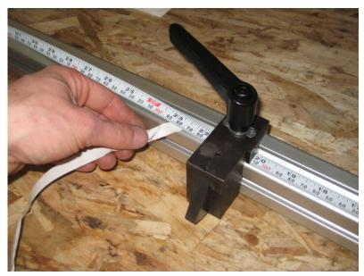
Slide the tape scale under the first Versa-Stop block and line up the indicator on the Versa-Stop block with the known location/measurement on the tape scale.
