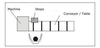
The only acceptable operator location in the work area is standing in front of the control stand on the opposite side of the conveyor (see picture above)
