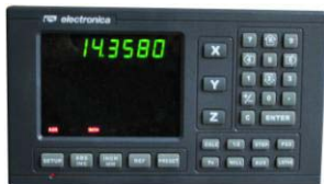
Fig 6. Digital Readout with 0.0002" resolution
