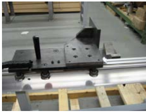
Fig 3. Movable carriage with cable track, handle and linear encoder
