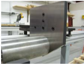
Fig 5. Moving steel V-stop with pipe loaded
